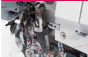
allows for easy threading in seconds— simply push the automatic threader up and then thread goes through automatically.
