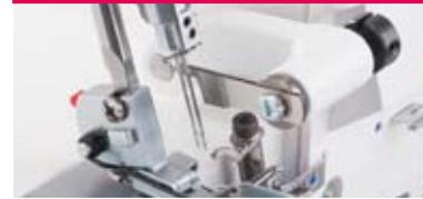
removes the upper knife so that threading is made safer and easier.
