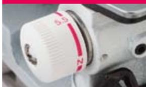
adjusts the lower knife quickly to change the width of fabric in the seam allowance, for perfect seams and rolled edges.
